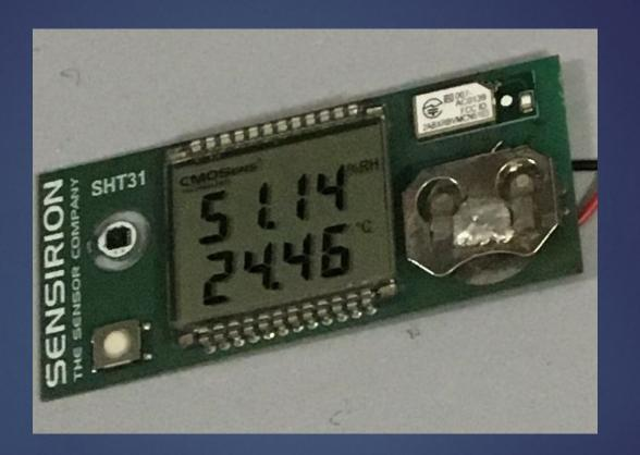
A single PMFC can supply a temperature and humidity sensor perpetualy
